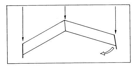
The above diagram shows a positively swept wing yawed slightly to the left. Notice that if the tip fins are toed in just a couple degrees then the right fin tends to correct the yaw. The left fin would similarly correct a yaw to the right. No drag penalty would be incurred at low yaw angles (compared with a flat plate mounted at 0 degrees) if the symmetrical airfoil used is chosen carefully. A list of possible sections is included at the end of this column.
