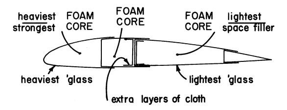
"The important thing to remember is that the shear web have sufficient strength to carry the compression loads tending to make the top and bottom surfaces touch."
