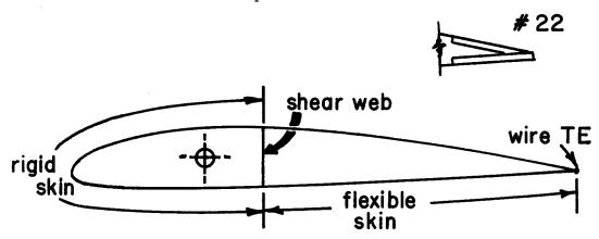
"If a wing were to be constructed as shown above, with a D-tube leading edge having a skin rigid enough to carry the shear load and a rear portion consisting of a flexible (Monokote) skin and a wire trailing edge (ala WWI airplanes) the structural axis could be at the C/4. The weight also could be forward so that we could have a very flutter resistant design.
