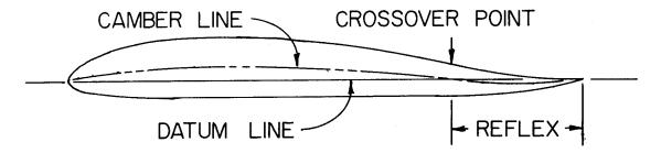
Notice the camber line and the fact it crosses over the mean chord line at the 75% chord point. The resulting section, the Clark YS, is an inherently stable airfoil because, contrary to what occurs with a normally cambered section, the center of pressure moves forward as the angle of attack decreases, and more rearward as it increases. Sections with greater camber will require more reflex in order to be made stable.
