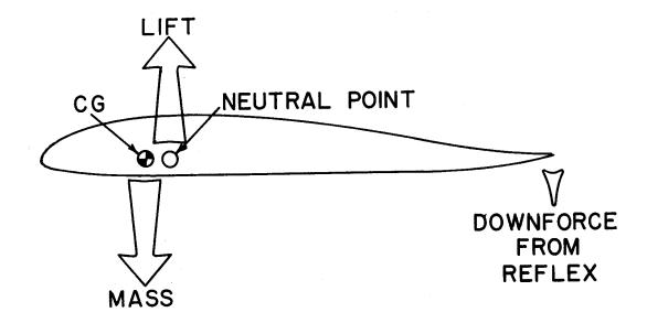
In trimming our plank, we place the CG ahead of the neutral point, thus producing a constant nose down force. When the CG is placed at the point where the nose down force can be exactly balanced by the aerodynamic downforce produced by the reflex in gliding flight, the airfoil is dynamically stable.
