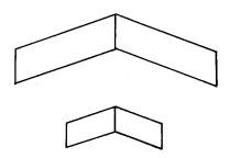
By simply moving the horizontal stabilizer halves to the wing tips we come up with a tailless planform.
