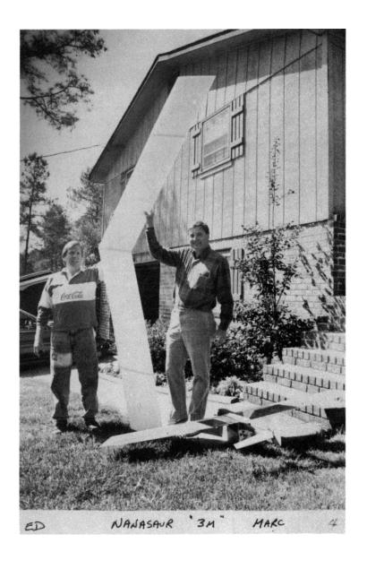
attack is changed. The use of the Eppler airfoils is important to limit the pitch sensitivity on a flying wing. I found the airfoils in Chuck Anderson's airfoil program and ordered the IBM version of the software. B' advised I use the E 222 at the root and the E 230 at the tip with 3 degrees of negative twist (T.E. raised) for thermal flying. I decided to use the E 222 for the root, transitioning to the E 230 at the tip.
