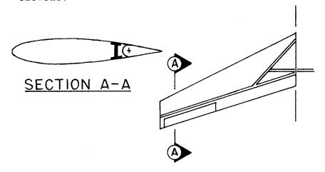
When the spar is placed to the rear of the airfoil it counteracts the torsion produced by the bending of the wing and the angle of attack of the tip is much more resistant to change. A fully sheeted foam core wing with this type spar system is very resistant to flutter even without winglets. A retrofit of this spar system would be very difficult in an existing 'wing, but what better reason to build a new one?
