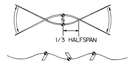
Before a remedy can be prescribed we must find the reason for the flutter. Take a piece of sheet balsa and extend 3/4 of it past the edge of a table. "Sweep" the sheet to some angle relative to the table edge, say 20°, and place a flat object, like a book, on the end of the sheet which is resting on the table. If you now lift or depress the free end of the sheet you will see an interesting thing happen; the effective angle of attack of the tip changes, as shown in the next drawing.
