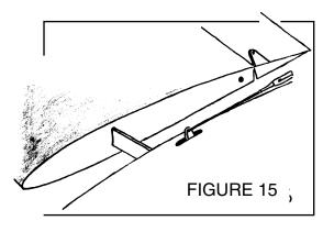
the separation point. Needless to say, the steel wing blade should not be inside the receptacle for this procedure.
