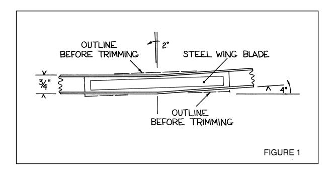
wing blade thickness) is used for the remainder. From the drawing we find the width of our plywood joiner before trimming must be at least 7/8" when the blade is centered within the structure. This width allows for some trimming of material upon completion of the basic structure, but minimizes waste. The receptacle length should be slightly longer than the steel blade to allow for end caps.
