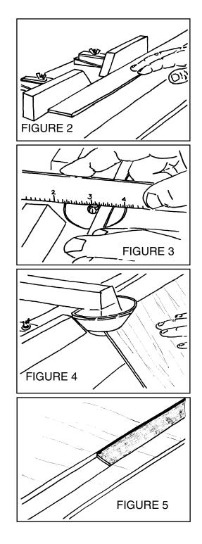
Now measure across the 1/8" plywood to the predetermined width of the untrimmed joiner assembly See Figure 6.
