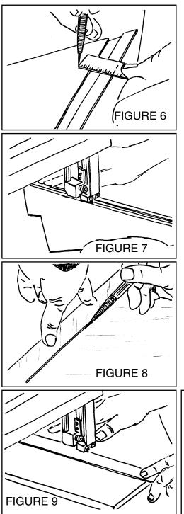
Place the completed piece on the 1/16" plywood. See Figure 8. Align the free edges and mark the 1/16" plywood using the 1/8" plywood as a straightedge. Remember, the strongest structure is obtained by orienting the grain of this face piece perpendicular to that of the routed piece.
