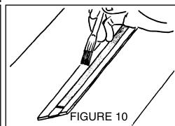
Align the assembly carefully and weight it for a good bond. Refer to the cutaway sketch, Figure 11, and the end view, Figure 12. When the epoxy is cured, grasp the free end of the steel wing blade with pliers and pull it out of the plywood assembly.
