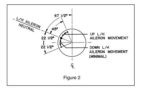
A rigid mechanism which overcomes these failings was submitted by our Minnesota friend Bill Kubiak. This system, presented in the September 1992 issue of *RCSD*, uses stiff pushrods and relies on servo wheel geometry to achieve differential action. This set-up is shown in Figure 2. When properly built, the mechanism allows no extraneous rudder movement, as the rudder is locked in the neutral position by the servo wheel. This rigidity makes the system less likely to flutter.
