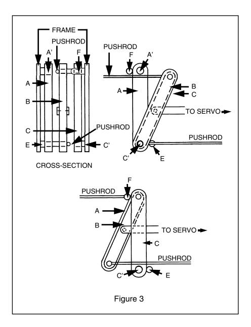
It should be noted the geometry of this walking beam magnifies the movement of the servo pushrod - a lever effect which places a proportionally larger load on the servo - so care should be exercised in the choice of the servo used. By adjusting the placement of pins E and F and the control surface pushrods, it should be possible to create a situation where the control surface is locked in the neutral position by a "toggle-over-center" action.
