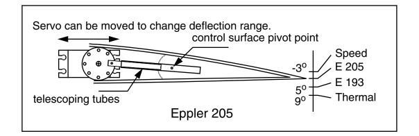
The diagram shows the component layout used within the wings of *Onnozel*, a "noseless" V-tailed sailplane designed for F3B. As you can see, the range of deflection for camber changing is just  $12^{\circ}$  — three degrees up and nine degrees down — but the total range of deflection is greater. The control surface can be moved in very small increments while being held rigidly in position at all times.
