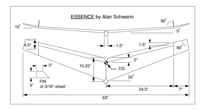
out from the root to the fins, and the roll rate is excellent. A minimal fiberglass keel provides a hand hold and houses and protects all of the radio gear. Total weight is 17 ounces, but with an area of 450 in $^2$ , the loading is down to 5.44 oz./ft $^2$ .
