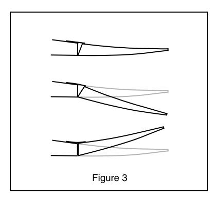
After building several Blackbirds of various sizes, we noted they all shared a common fault. When flying in a straight line, alternating left and right aileron input did not produce rolling motion. Rather, the wing would simply oscillate around the yaw axis.
