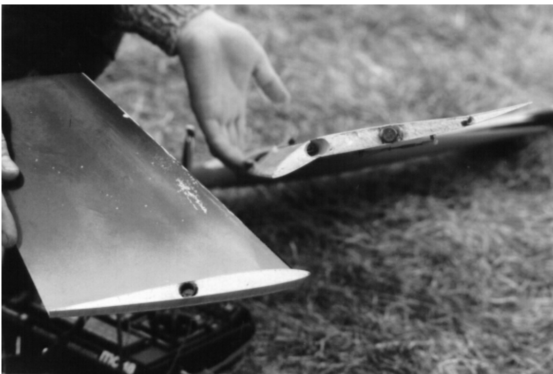
Photo of Joined 2, with winglet removed, showing moveable leading edge, elevon, and winglet mounting method. EH 1.0/7.0 airfoil is used.
