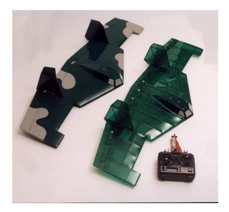
Over the last six months I have made four flying wings: a 60 inch foamy utilizing a conventional swept back wing, and three others having this wing platform. Two of the latter wings have a wingspan of 50 inches,  $500 \text{ in}^2$  wing area, a fully symmetrical airfoil, and weights of 14 and 23 ounces. Due to the successful flight characteristics of these first two, I decided to make something big.
