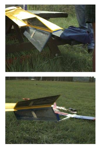
With the improved visibility offered by the addition of winglets, flight testing began providing legitimate feedback. Flight characteristics continued to improve as the CG was moved aft, the tow hook was relocated, and radio mixing was reorganized.
