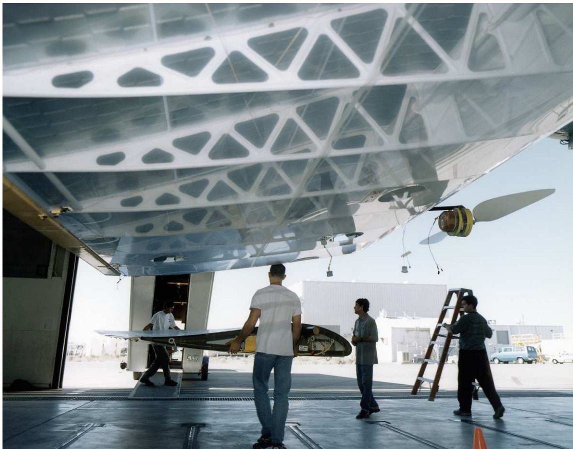
Dryden Flight Research Center EC96-43765-8 Photographed November 1996 LIGHT AS A FEATHER--Technicians easily lift a 20-foot wing section during assembly of the Pathfinder solar-powered aircraft. NASA photo by Dennis Taylor
