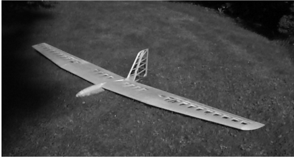
The completed Raven airframe, ready for covering.
