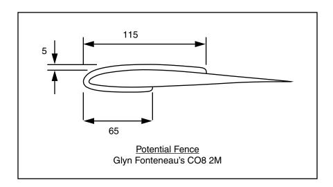
installation of potential fences often dramatically improves controllability at high lift coefficients. Watch for a comprehensive article on potential fences in a future "On the 'Wing..." column!
