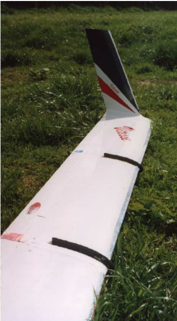
Closeup of the winglet and wing fences, Dave and his Vitesse. Both Vitesse models are well behaved and fly magnificently.
