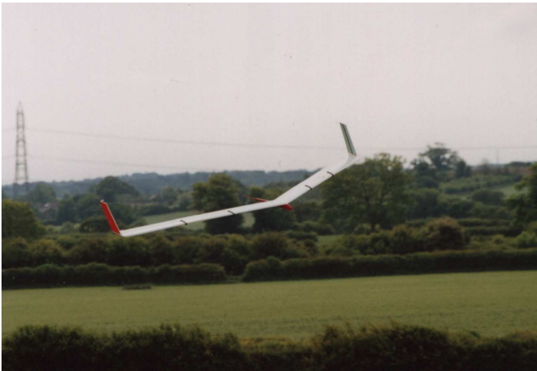
Glyn Fonteneau's Vitesse on the ground and in the air. Glyn, like Dave, added double sets of wing fences and saw an immediate performance and handling improvements. Glyn did not add the sub-winglets to make a C-wing configuration.
