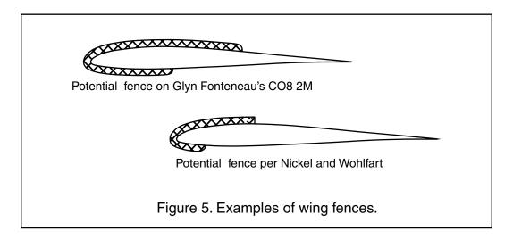
shown to be very effective at controlling adverse stall behaviors and maintaining control surface effectiveness at high angles of attack. Installing two fences on each wing panel, at 1/3 and 2/3 of the semi-span, has been found to be effective on high aspect ratio wings with steep sweep angles.
