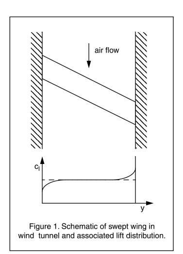
From a slightly different perspective, by removing the walls and attaching a "mirror" wing panel to either the left or right end of the existing wing, we have a complete wing, swept either backward or forward, and an associated lift distribution as depict in Figure 2. We can consider a wing fence to be aerodynamically equivalent to a tunnel wall. This effect is demonstrated in a more comprehensive way in Figure 3.
