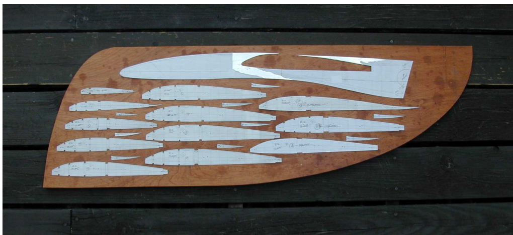
The R-2 templates: fuselage sides, wing, elevator, and aileron ribs all rest on the 3/4" plywood form for the fin leading edge (left) and wing leading edge (bottom right).
