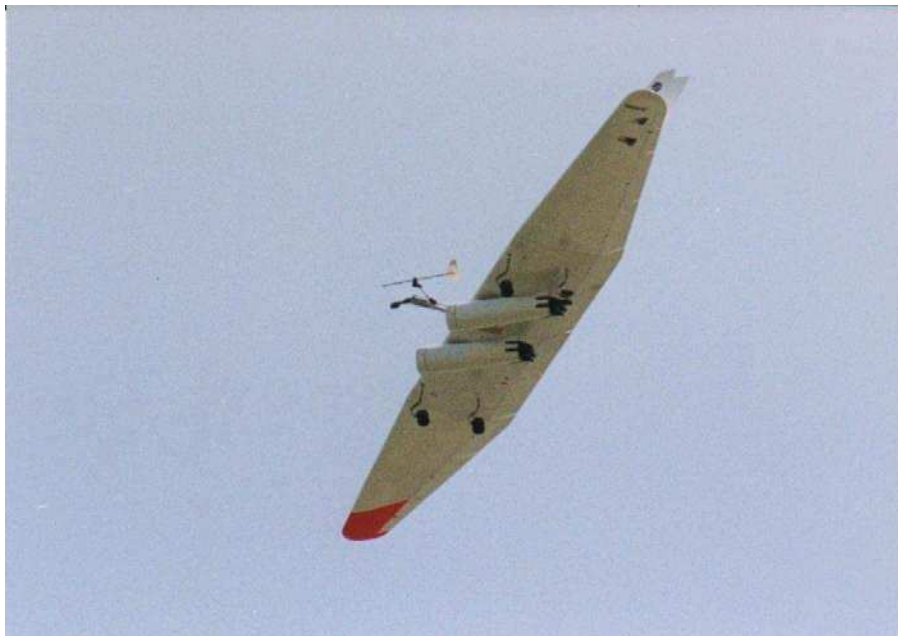
The oblique wing in flight. The yaw/angle of attack vane indicates the direction of flight. Eighty pounds and a twenty foot wing span moving through the air at a good clip...
