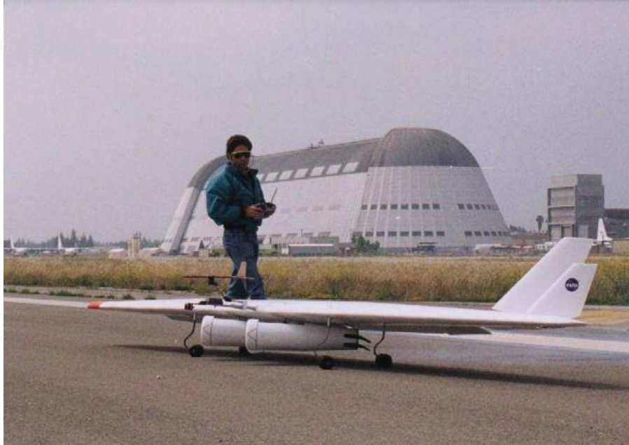
Steve and the oblique wing. Twin engines, twin verticals, dual wheel sets all around. The sensors for angle of attack and yaw can be seen above the starboard engine inlet.
