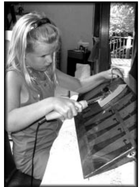
The wings were covered in Monokote transparent green.
