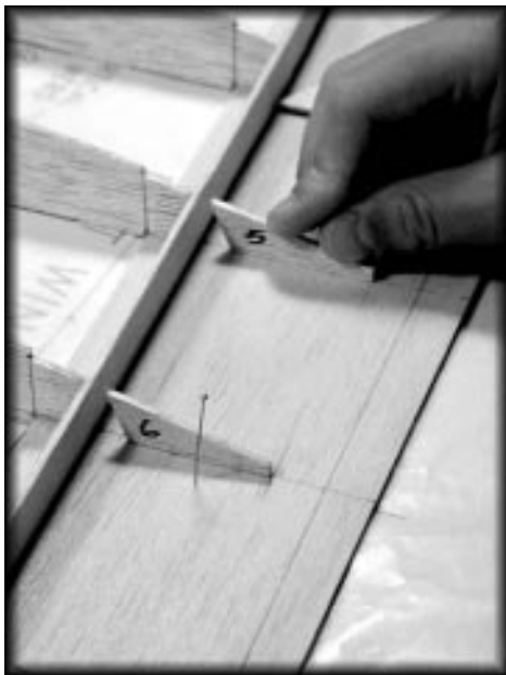
The aileron ribs were cut from the wing ribs, and the ailerons are fully sheeted.
