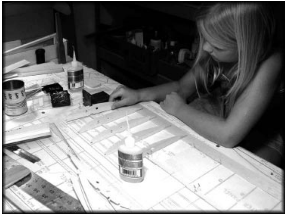
I used machinist blocks to make sure the ribs were glued in straight.
