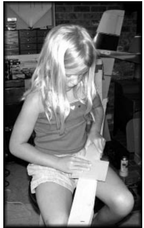
I painted the fuselage. I sprayed on a coat of primer first, and sanded it down with a foam sandpaper pad. Then I sprayed on two coats of white.
