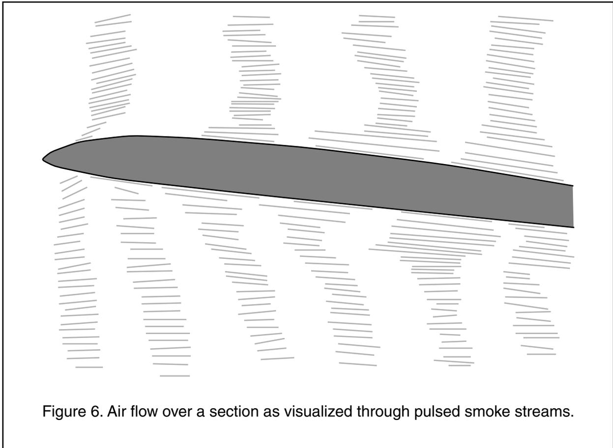
Figure 6. Air flow over a section as visualized through pulsed smoke streams.
