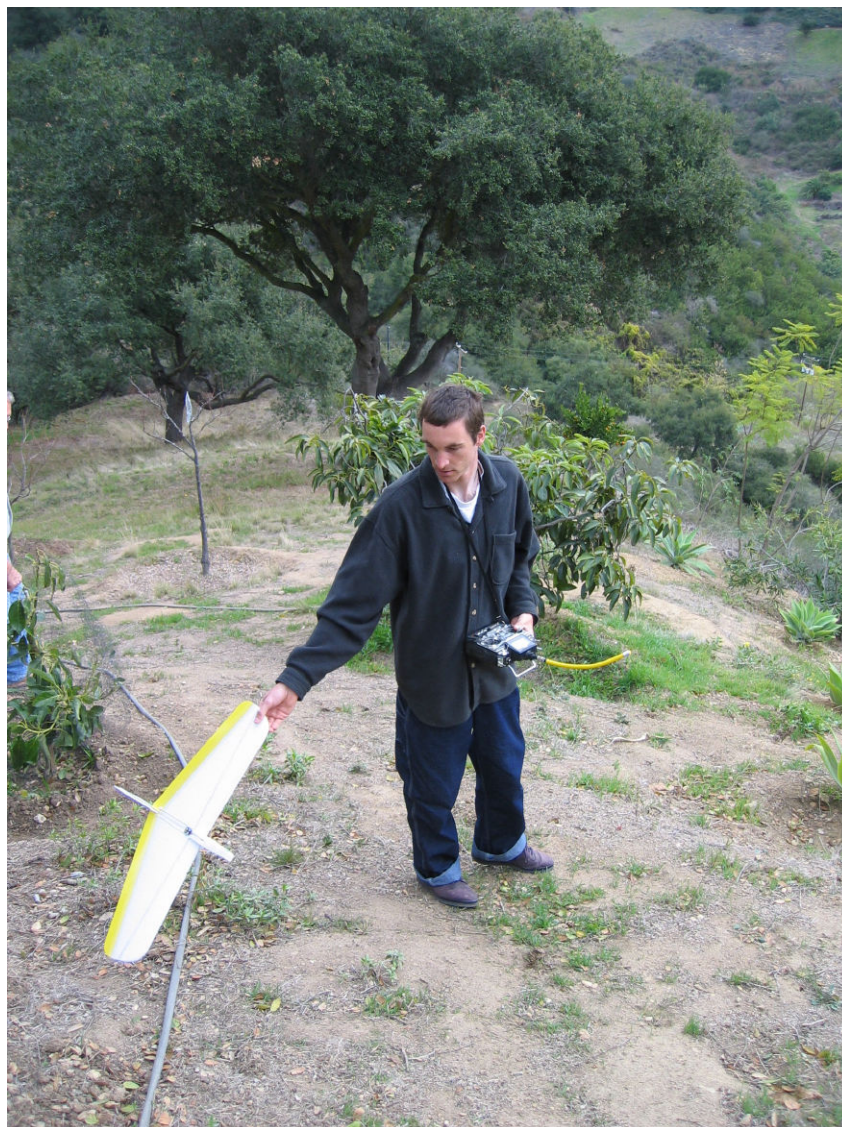
Michael ready to launch his Alula on its maiden flight. Because of its light wing loading and forward swept wing, Alula excels in light "slermal" lift.
