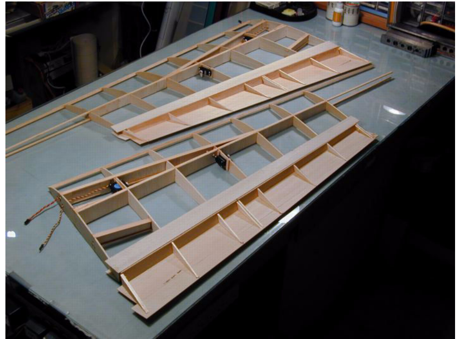
Right: Wings under construction. Of particular note is the main spar system, composed of two subassemblies, which will be tied together by the upper and lower surface D-tube sheeting. Elevator servos are mounted to Rib 2, aileron servos to Rib 4. Still a lot of 1/16" sheeting to go!
