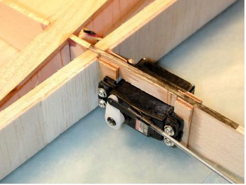
Upper left: The elevator servo (Hitec HS-425BB) is installed between the two spars. The pushrod slot is cut into the webbing of the lighter rear spar, so the reduction in overall spar system strength is relatively small. The leading edge sheeting will completely enclose this servo, so we're heavily relying on Hitec reliability. We can always remove the sheeting if the servo fails.
