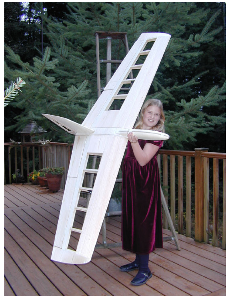
Granddaughter Alyssa shows off the framework of the Redwing 2M . Weight at this point, ready to 'glass and cover, with all servos installed, is 50 ounces.
