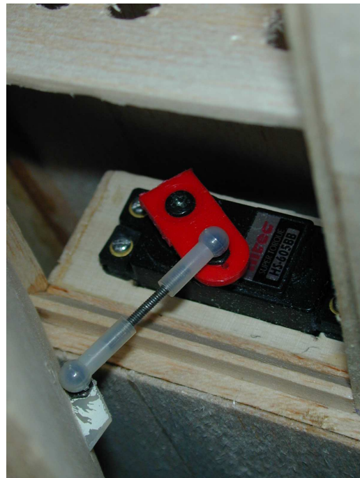
A photo of the reversed servo in place in our newest Blackbird XC. The flap is deflected to 45 degrees. Notice the high strength output arm which comes with the servo. (The three unused arms have been cut off.)
